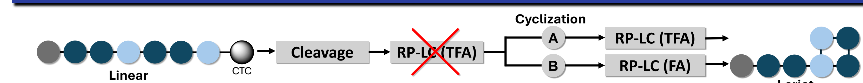
Figure 6. Post-SPPS Workflow. Elimination of linear RP-LC purification step allows rapid progression. Sequences that required Cyclization condition B were purified with formic acid buffer to avoid ring breakage.
